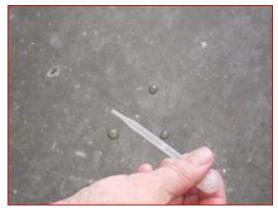
Water Droplet: Pipette Application Note no immediate absorption
