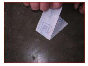
Cross Hatch Test – No visible cuts or flaking on the back of the tape
